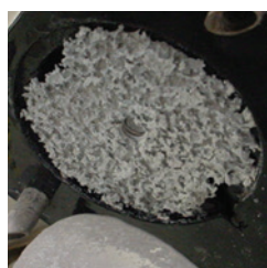
Unprotected and premature transom & outdrive zinc loss
