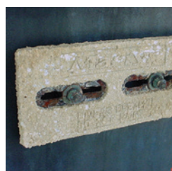
Unprotected and premature transom & outdrive zinc loss
