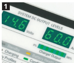
1 Dual Digital Displays and Power Output Bar
