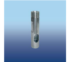
▲ PRM280 Electropolished AISI316 stainless adaptor 1" BSP x 11 tpi male to 1" x 14 UNS female, with slot for cable
