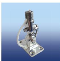
▲ RA107SSFME 4 Way ratched mount in stainless steel, locking by clamp, with cable slot, 1"x14 standard thread
