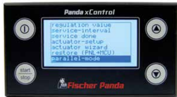
All generators with xControl can operate in parallel
