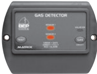
600-GDL Same features as the 600-GD, with the ability to switch a valve on. It contains a unique "Pulse & Hold" circuit within the detector. This allows the valve to be pulled in at 12V and then once energized it will step down to hold the valve in place. This reduces power consumption and heat while the gas is turned on.
