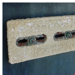
Unprotected and premature transom & outdrive zinc loss
