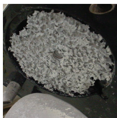
Unprotected and premature transom & outdrive zinc loss
