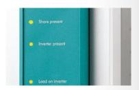
Read-out of the basic functions on the display, including indication of available power source, generator, grid power or inverter and 'load on inverter' function.
